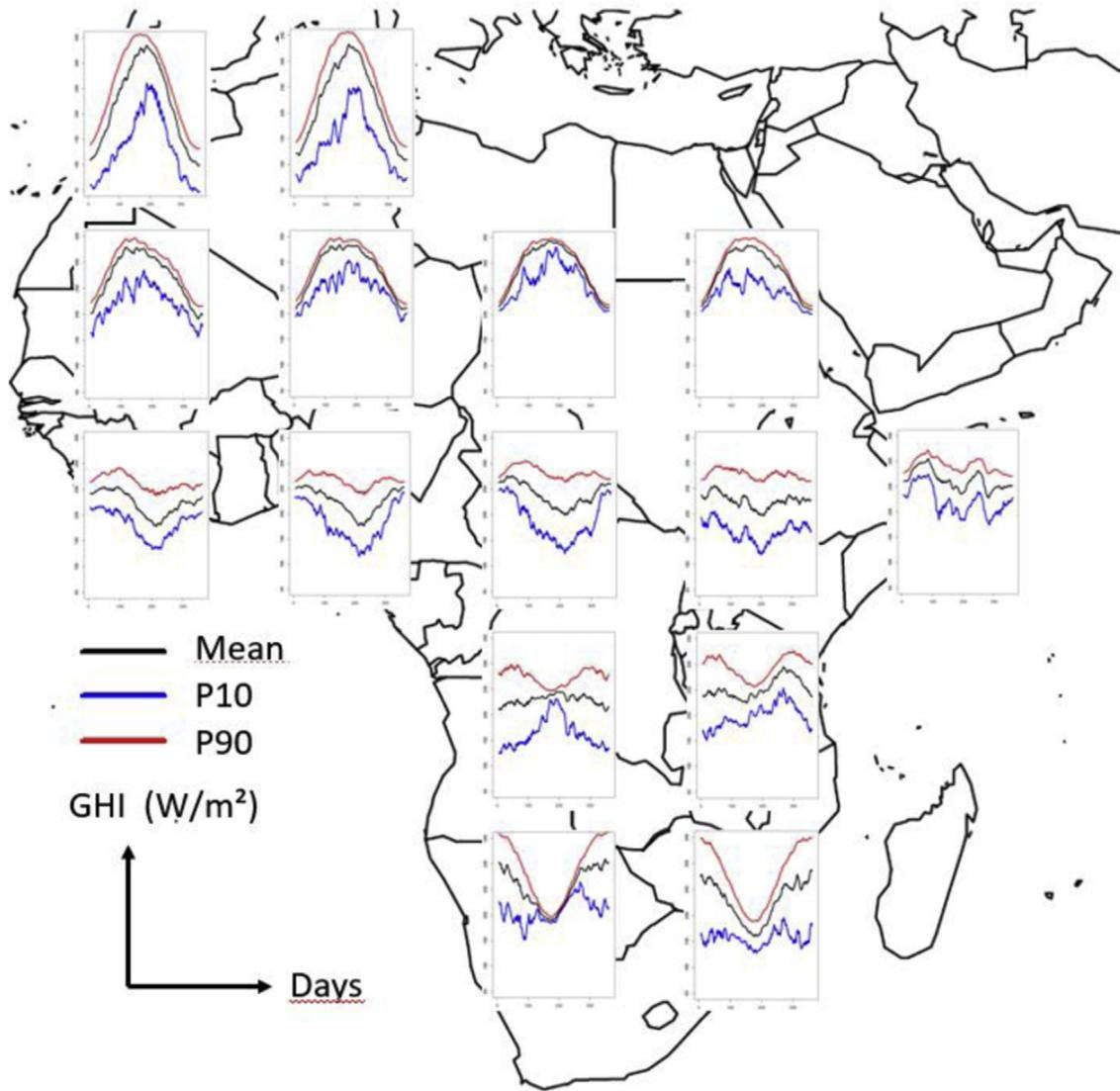
**Fig. 3.** Variability of daily GHI values [ $\text{W}/\text{m}^2$ ] for 15 SARAH grid points in different African climates. Mean value (black), 10th (blue) and 90th (red) percentiles of daily GHI for each calendar day (1995–2015 period). See location of grid points in Fig. A1 of Supplementary Material. Scale for the y-axis: from 50 to 350  $\text{W}/\text{m}^2$ . (For interpretation of the references to colour in this figure legend, the reader is referred to the Web version of this article.)
