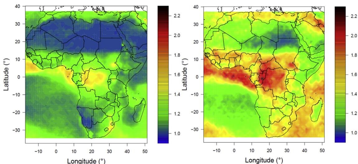
**Fig. 10.** Increase in low percentile values of daily GHI when estimated over a 2 days moving average window. Left: ratio between P5 values calculated respectively from 2 days mean GHI data and from raw daily data. Right: the same with P1 (percentiles obtained for period 1995–2015).
